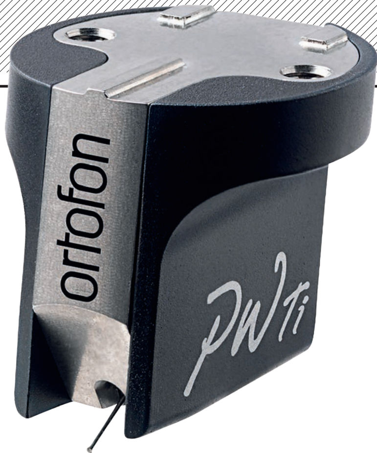
LEFT: The two-part titanium body with alloy 'overcoat' includes threaded mounting holes, but note the three points of contact on the cartridge top. The exposed cantilever demands caution but cueing is made much easier
